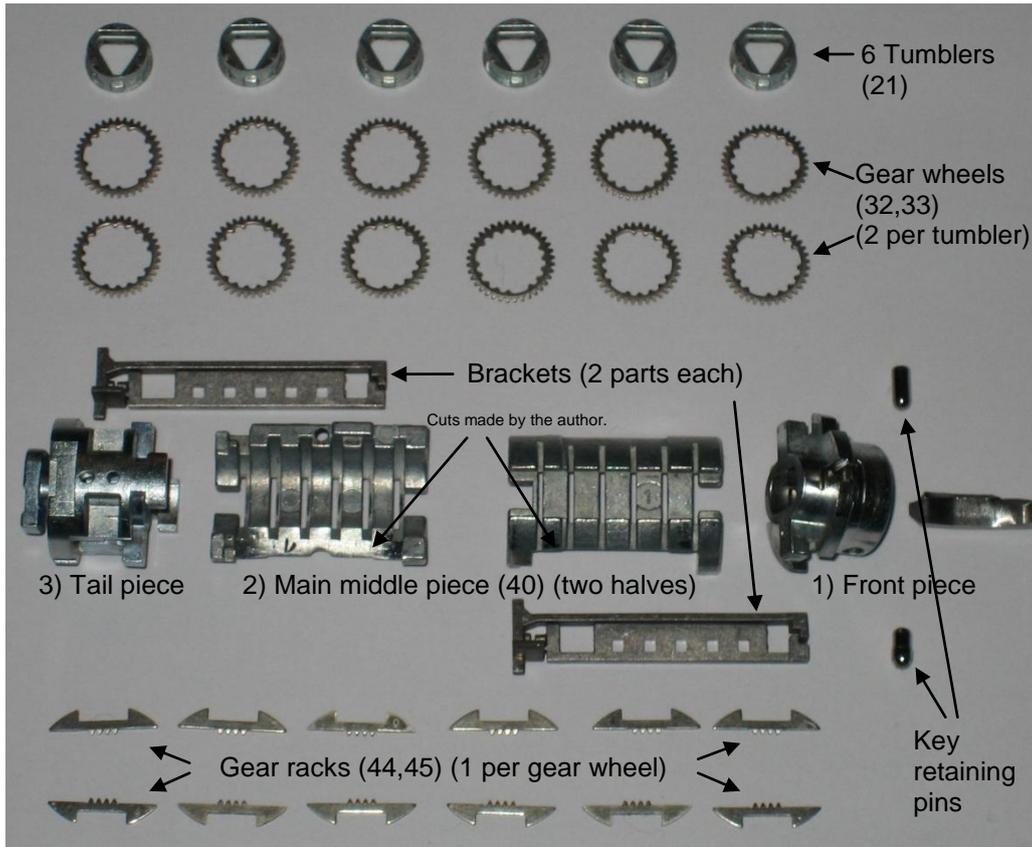
Fig. 6: The parts of the rotor.
