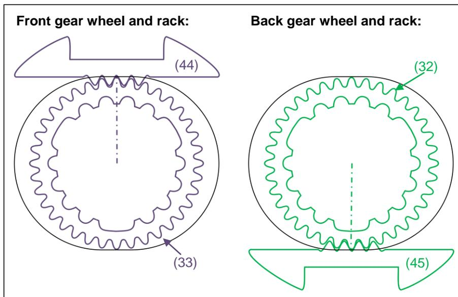
Fig. 9: Gear wheels in the middle (M) position.
