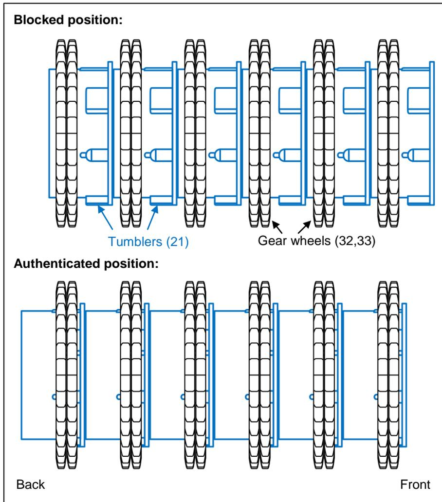
Fig. 7: The stack of tumblers – side view.
