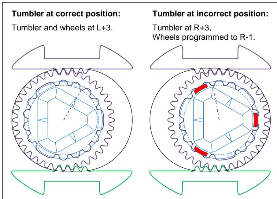
Fig. 11: Correctly and incorrectly positioned tumblers – view from the front.
