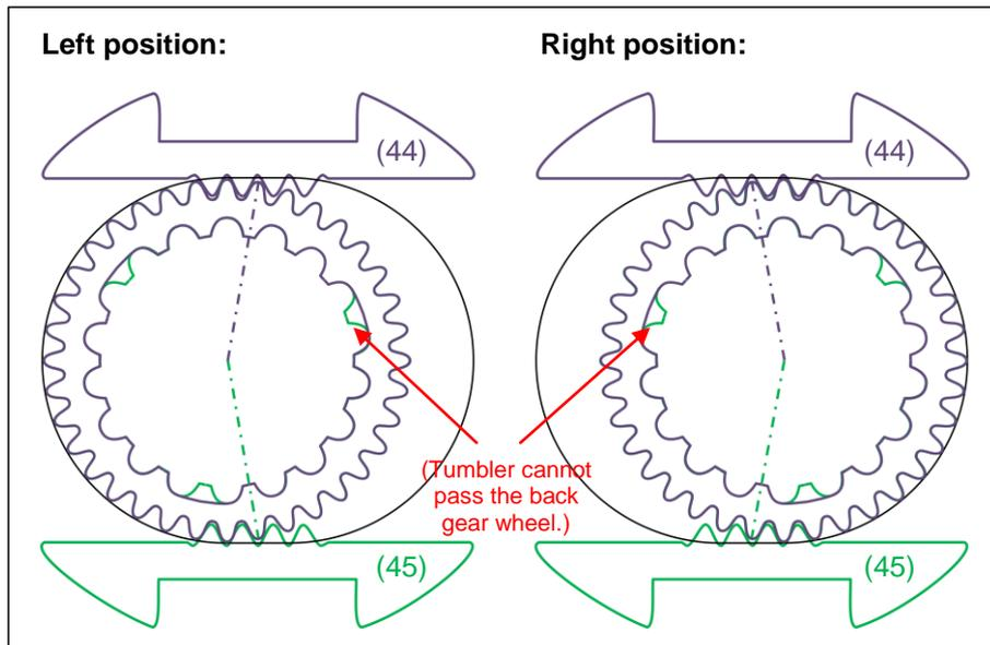
Fig. 10: Gear wheels moved to the left (L) and right (R) positions.
