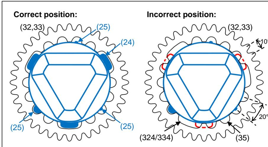
Fig. 8: Tumbler and gear wheel – view from the back.
