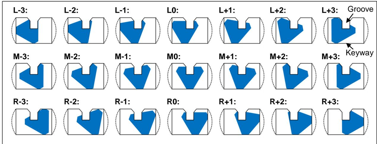
Fig. 14: Twenty-one possible key cuts – cross sections, view from the bow.
