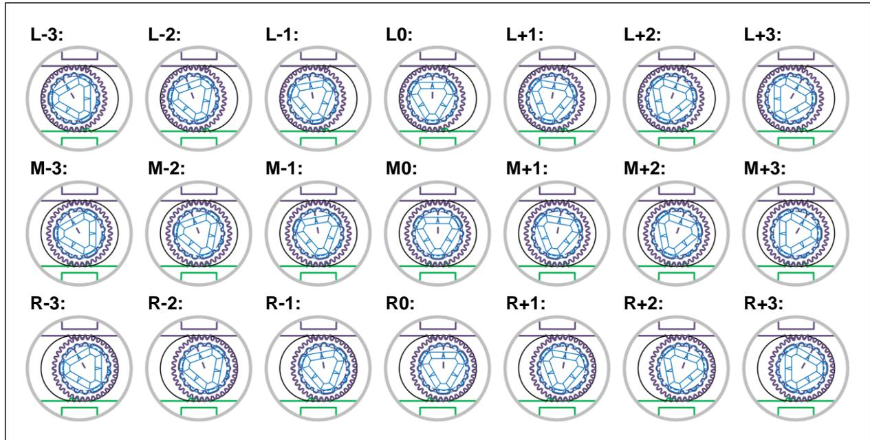
Fig. 12: Twenty-one possible positions for each tumbler.
