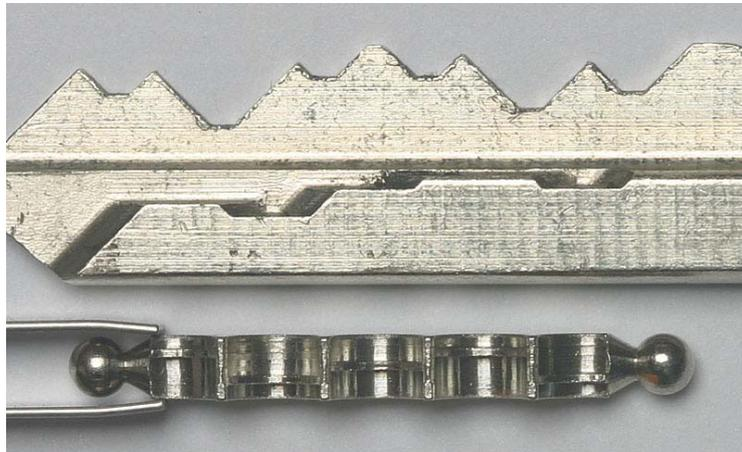
*Note: During the photo shoot, I mixed up the side bars. I wanted to make a picture of the streamlined side bar with the matching side bar (cuts 32454). However, I took the wrong side bar and used the side bar with the side bar cuts 24324. The key has the side bar cuts 32454. For understanding how the cuts in the side bar profile work, this picture is fine.*
