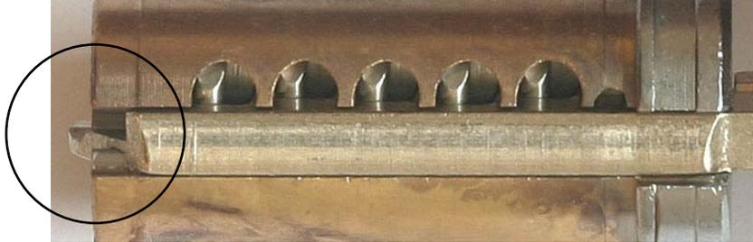
**Details of the bottom of the Twin V10 keyway with the key inserted**
