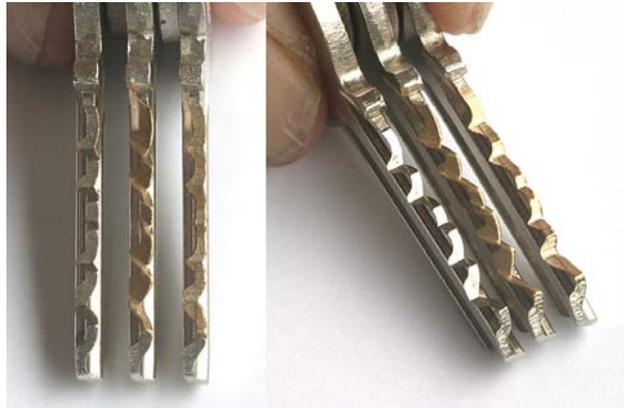
***Original key (left), copied key with angled cut, which fits (middle), straight cut key from angled cut key, does not fit (right)***
