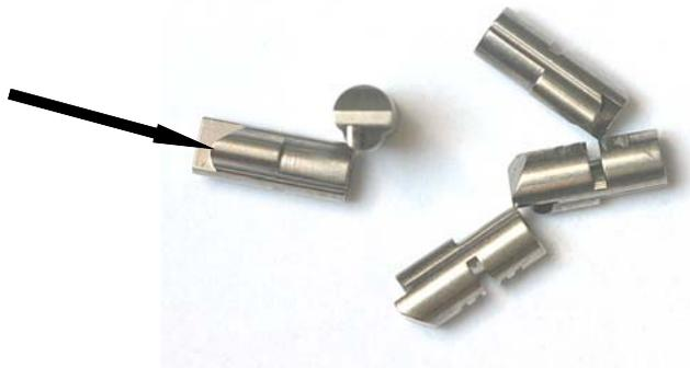
**Detail of the side pins in the Twin Maximum**
