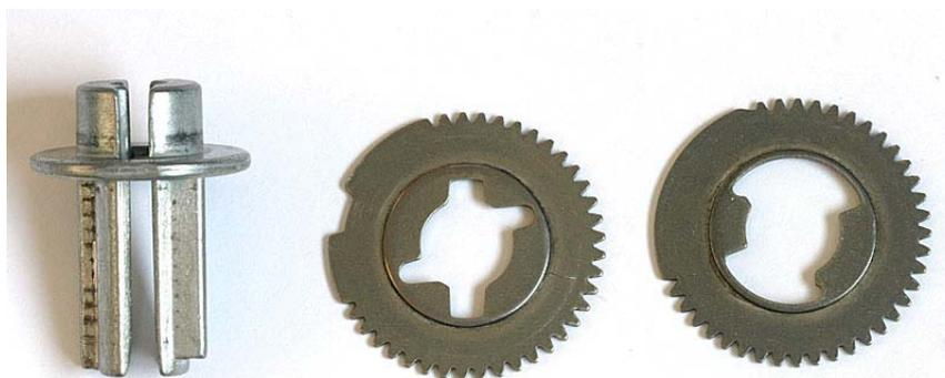
***Parts in first wheel package, Curtain, Drive wheel, Lever wheel.***
