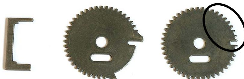
**Parts in second wheel package: Fence, Fence drive wheel, Blocking wheel,**
