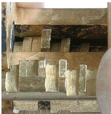
***Ava wafers in the locked position, in combination with the correct key***
