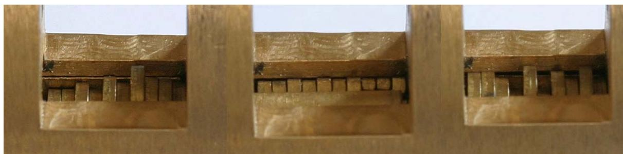
**Sliders in locked position, open position and false key position**
