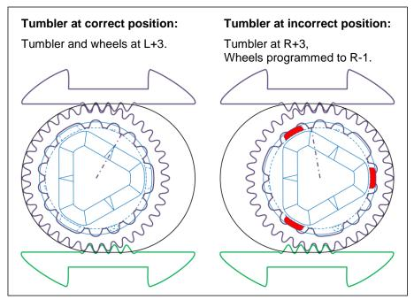
Fig. 11: Correctly and incorrectly positioned tumblers – view from the front.
