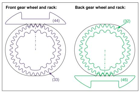
Fig. 9: Gear wheels in the middle (M) position.
