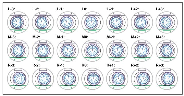
Fig. 12: Twenty-one possible positions for each tumbler.
