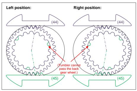
Fig. 10: Gear wheels moved to the left (L) and right (R) positions.
