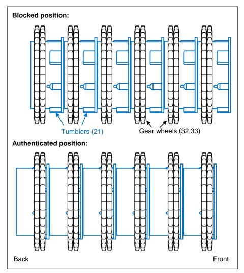
Fig. 7: The stack of tumblers – side view.
