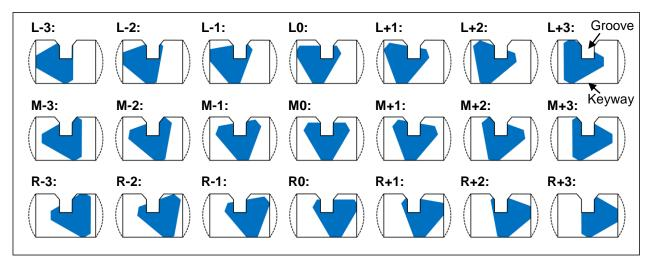
Fig. 14: Twenty-one possible key cuts – cross sections, view from the bow.
