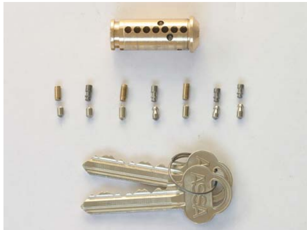
Parts in an ASSA 7-Pin Cylinder
