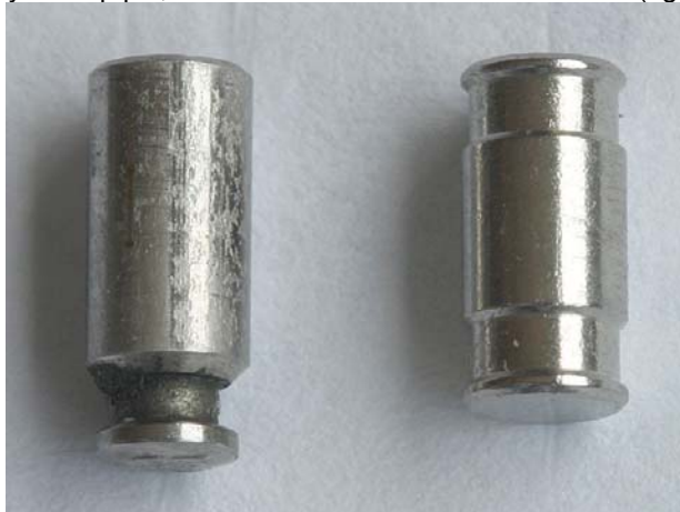
Spool driver pins used in a Twin/V10 Instruction and Demo cylinder
