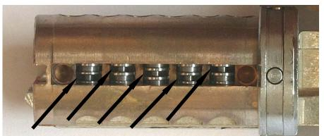
Details of the groove in the plug of the Twin 6000 where the locking bar drops in
