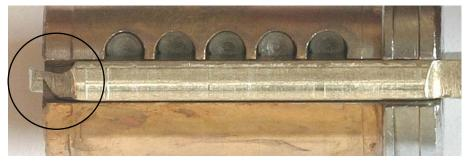
**Details of the Twin 6000 bottom of the keyway with the key inserted** Note: The specific tip of the key in this system. Later in the article you can compare the tip of the key with the other systems. The reason for the different shape of the tip is probably the ramp which makes first contact with the side pins.
