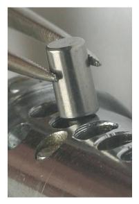
**Top pin A in the "locked" position in a counter mill** Note: When picking to release the "locked" top pin you have to rotate the plug back most likely causing all the other top pins to fall back too.
