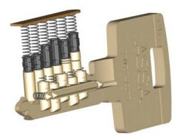
Details of the working of the side pins in combination with the side bar.
