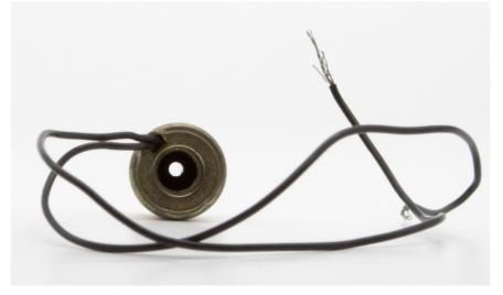
A metal rod is placed inside the coil. The thick end of that rod sits inside the coil; the thin end extends into the cylinder through the hole. The plastic cover prevents the rod from falling out when the magnet is off.
