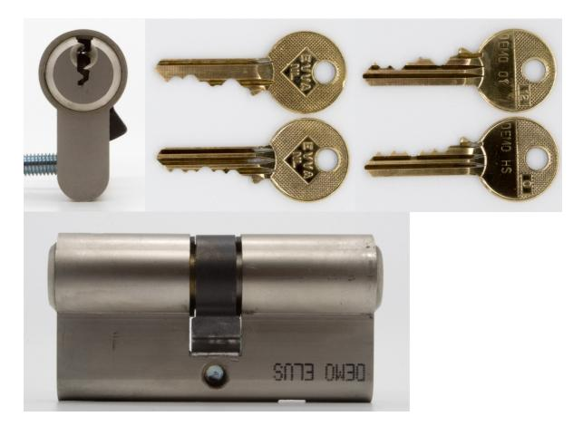
The NL key with KG profile does not fit in this ELUS cylinder and the DEMO 01 key with 12 profile does not fit the NL cylinder. The master key fits in both cylinders. This indicates that the ELUS is a variant of the EVVA NL system.
