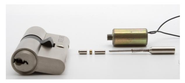
In the picture above, all parts are shown. The moving rod enters the hollow driver pin and hollow master pin when the electromagnet is activated. It reaches its highest position when it touches the solid key pin and it will stay in that position when the magnet is on.
