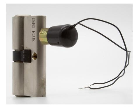
The device sticking out is a small electromagnet, screwed into the housing. You can see a plastic protective cover on the back of it with two wires coming out. The picture below was taken from behind the electromagnet (being the underside when the cylinder is mounted) with the plastic cover taken off. We can see that we are dealing with a simple coil with a hole in the middle. When applying a voltage to the coil, it becomes magnetic. The coil operates at 9 volts.
