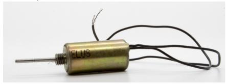
In the cylinder is a hole, through which the rod enters. If there were to be just this rod, it would go up through the housing into the plug, when the magnet is active. If the tip reaches into the plug, it blocks the shear line and prevents the cylinder from opening. The magnetic force is only moderate, so a key inserted into the keyway would very easily overcome the magnetic force and push the rod out of the plug into the housing, still being able to open the cylinder.
