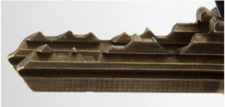
Looking closely, we can determine both keys have a different bitting depth on all of the five pin positions.
