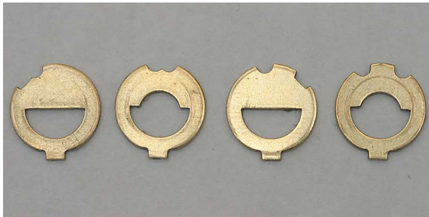
Masterkeysystem discs with more gates.
