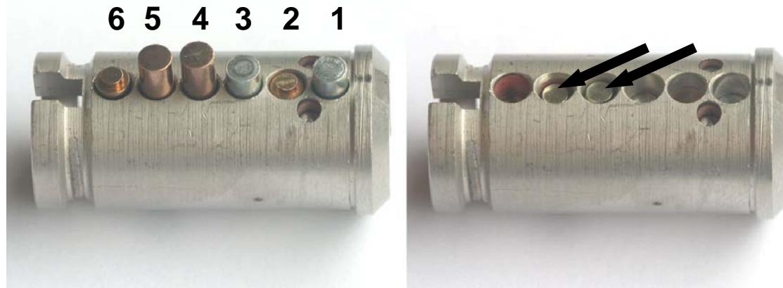
**Core / Plug with top pins and without top pins**
